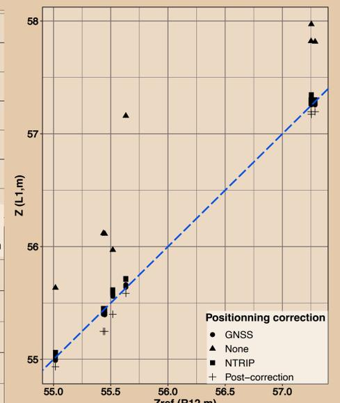
**Fig 3** : Comparative Analysis of GCP altitude measurements obtained by LiDAR L1 with various corrections and altitude measurements acquired by the trimble R12.
