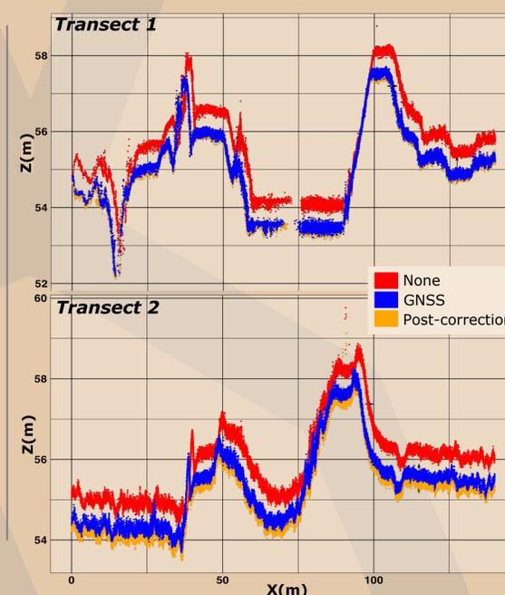
**Fig 2** : Topographic profiles derived from point cloud without correction (red), with correction (blue), with post-correction (orange)
